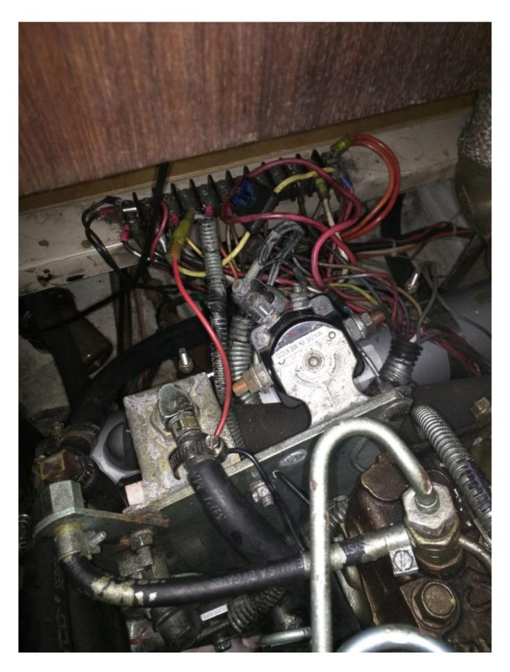
The wire with a resistor broke at one point and it seems to be the culprit for this issue
