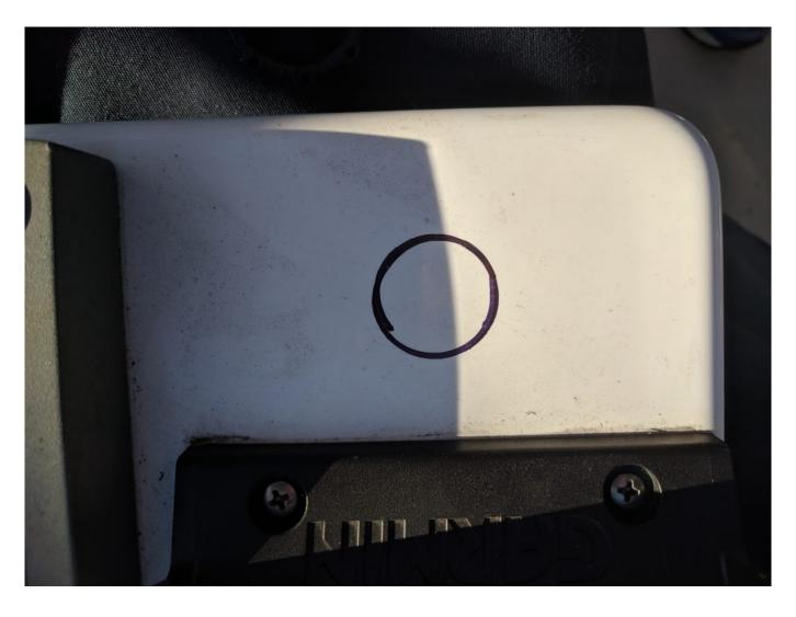
Use an  $1^{\prime\prime}1/8$  hole saw to cut the navpod after a first drill at the center of the circle.
