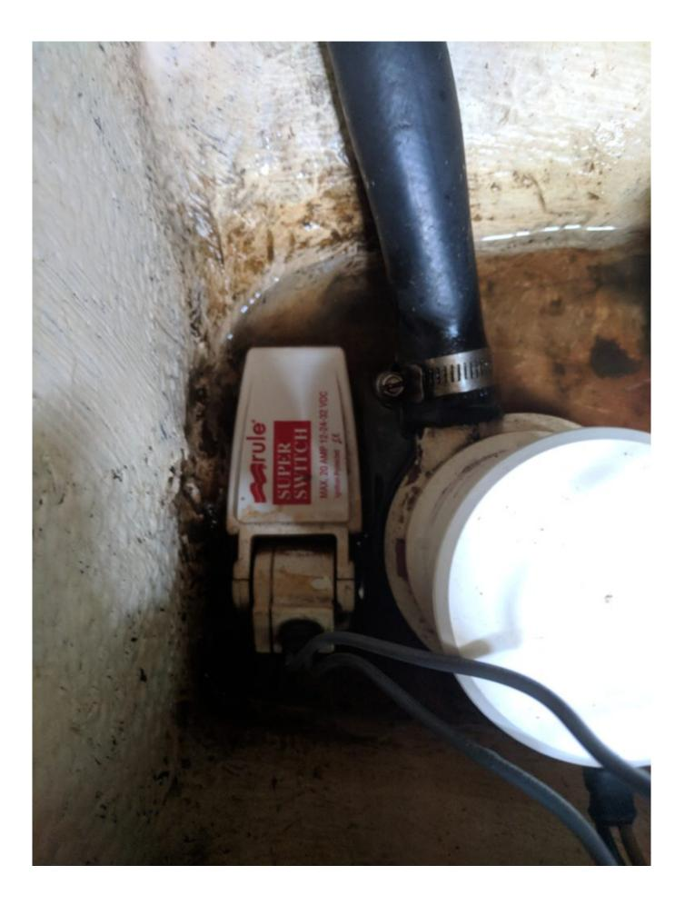
Corroded wires, after some troubleshooting and wiring the pump to by pass the switch, I was sure the issue was the switch.
