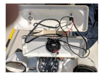
Time to investigate what is inside this NavPod, only the controller for the ST4000+ and one cable to power the Garmin GPS display.
